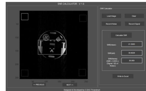
Figure 2. SNR measurement with a single-channel loop coil: axial slice of a phantom
