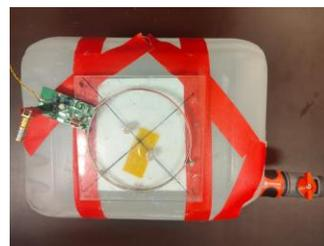
**Fig. 2:** Measurement setup using the flexible coil on the container phantom with a size of  $18.5 \times 14.5 \times 25.2$  cm<sup>3</sup>.
