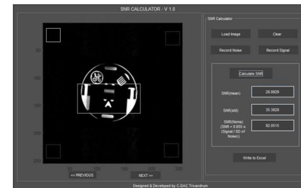
Figure 3. SNR measurement with 4-channel flexible surface receive coil: axial slice of a phantom
