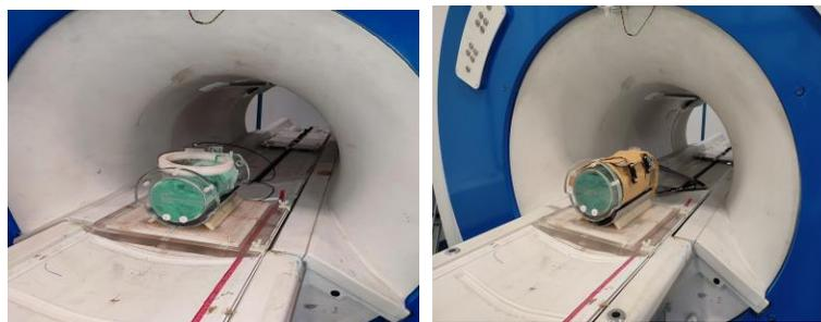
Figure 1. Left: MRI scan setup with single-channel surface receive loop coil (rigid) for phantom imaging; Right: developed ultra-flexible 4-channel receive coil wrapped around phantom
